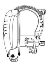
The body is equipped with an ingenious adjustable weight system, which allows the diver to adjust the center of gravity of NarmorX before the dive, depending on his/her body characteristics and water conditions.
